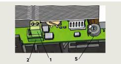
Fig. 11.2.4 115 Vac power switch
