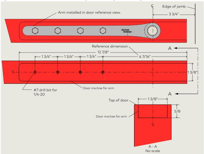
Fig. 12.2.3 Overhead center hung arm dimensions
