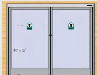
Fig. 9.5.2 Two way traffic, approach side
