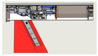
Fig. 12.5.4 Door bottom pivot on floor pivot bearing
