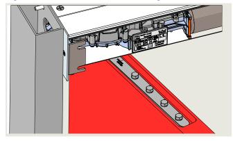
Fig. 12.5.8 Height adjustment wrench 08046540
