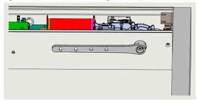
Fig. 11.8.4 Overhead arm at 70 degree position for door installation; LH inswing example
