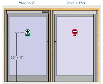
Fig. 9.3.3 One decal, two way traffic
