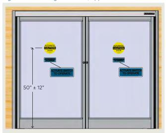
Fig. 9.6.2 Push/pull, door push, approach side
