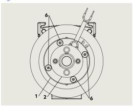
Fig. 21.4.6 Brake disc assembly removed from brake
