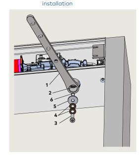
Fig. 21.3.2 Arm shown at 70 degrees for door removal and installation.
